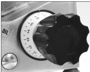
Precision adjustment of slice thickness.
