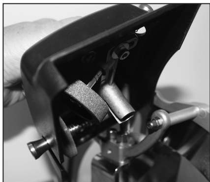
The integrated and removable sharpening device is simple and safe to operate
