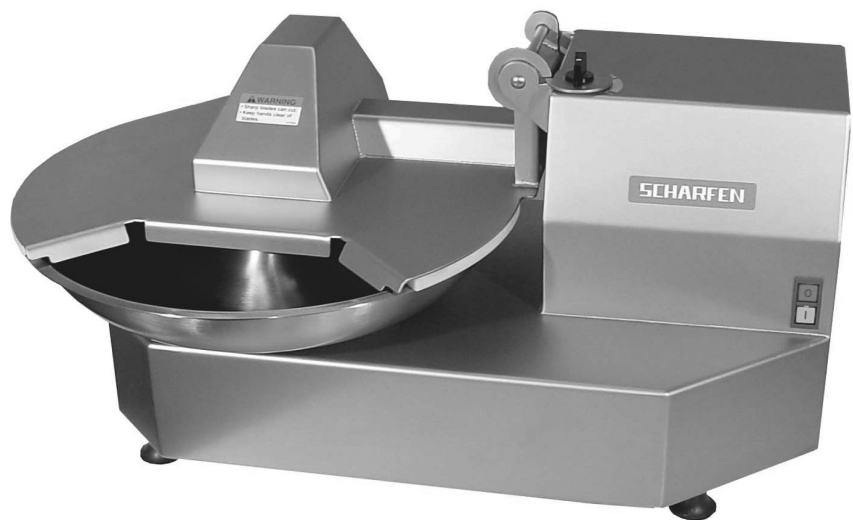
Safety interlock switch on bowl lid for greater operator safety
